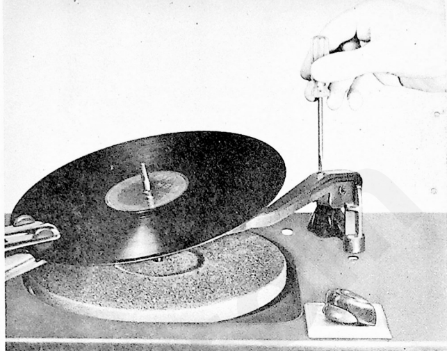
Figure 6—ADJUSTING TONE-ARM LIFT.
