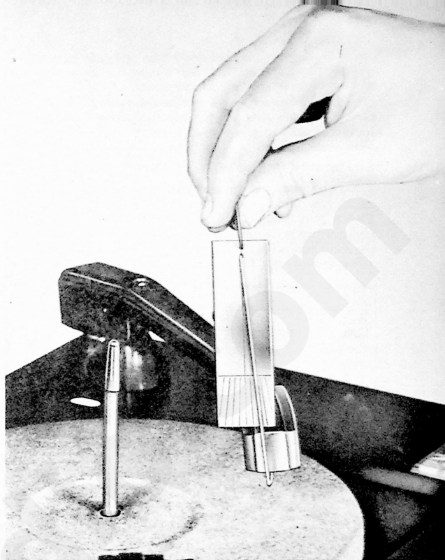
Figure 10—MEASURING TONE-ARM HORIZONTAL FRICTION.
